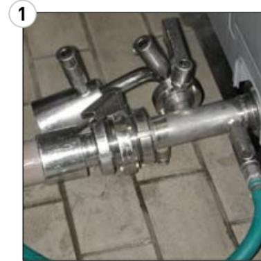
1 The discharging equipment is connected to the valve.
