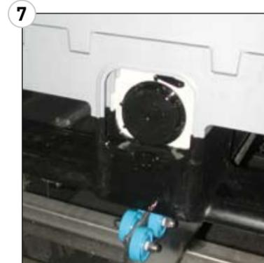
7 A cap is screwed onto the valve before the disposable liner is disconnected from the container.
