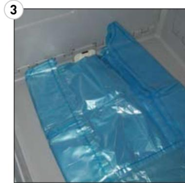
3 The liner is placed in the container with the valve fixed to the base.
