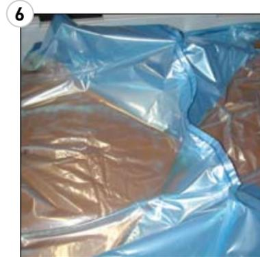
6 The liner is filled with liquid product automatically through the valve. No operator supervision required during filling.
