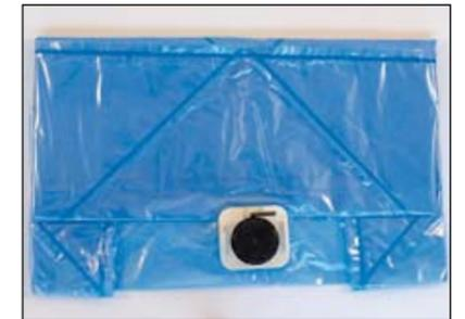
The three-layer liner bags are made with two inner layers of LLDPE and an outer layer of EVOH to give a good protection barrier. The valve is made primarily of polycarbonate, chosen for its excellent performance when heat treated.
