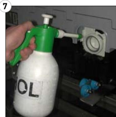
7 The outlet of the closed valve is sprayed to prevent bacteria from accumulating.
