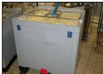
The CL 285BD is automatically filled from the top or via a bottom discharge valve.
